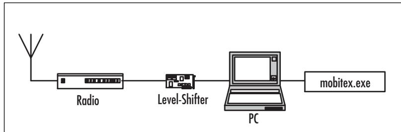
Simple circuitry is needed to convert the audio signal from the radio receiver into the proper levels for computer interfacing. I built the level-shifter hardware—some people call it a *POCSAG decoder* or *Hamcomm interface*—with a few dollars' worth of common components that we had lying around the lab. I plugged one side of it into my laptop's serial port and connected the audio output from the radio into the other side.
